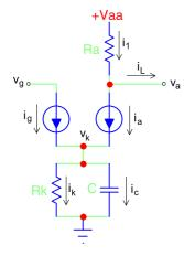
where  $v_g(t)$  is the voltage on the tube grid,  $i_g(t)$  is the current flowing into the grid,  $v_a(t)$  is the voltage on the anode and so the voltage at the output of the amplifier, and  $i_L(t)$  is the current flowing out of the amplifier into the load. The equations we are looking for are simply a law between these variables. Note that the load at the output and the de-
