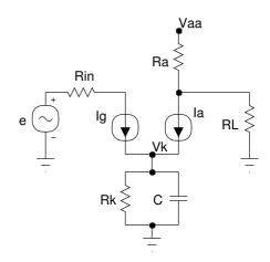
The voltage generator e(t) represent the signal at the input at the tube stage, so we call its value  $v_{in}$ . The output of the stage is  $v_a$ , the voltage on the load resistor  $R_L$ . The equations for this circuit can be easily written starting from the equations in the previous section and adding into the system the new relations between the input current and input voltage, and between the output current and the output voltage.
